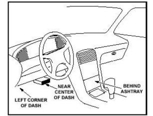
a label should be there telling location. For some Asian and European vehicles, the DLC is located behind the ashtray and the ashtray must be removed to access the connector. If the DLC cannot be found, refer to the vehicle's service manual for the location.
